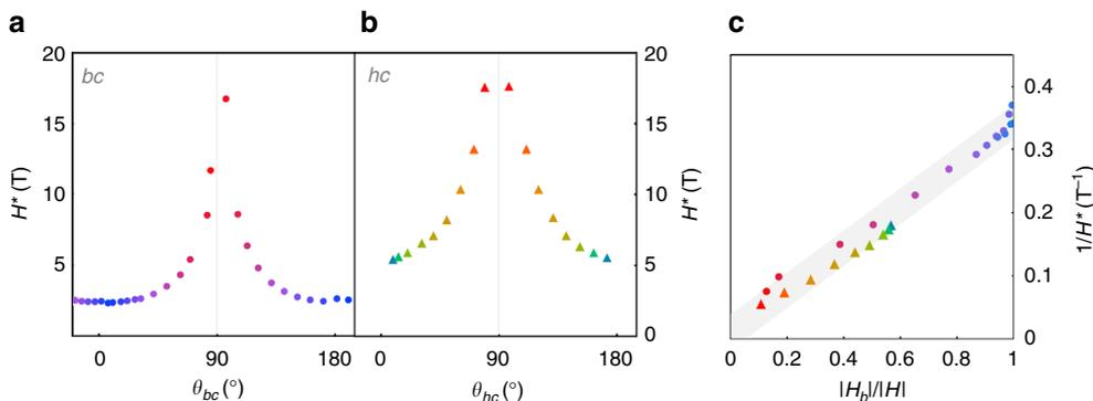
**Fig. 2** Angle dependence of  $H^*$ . **a**  $H^*$  vs. rotation angle  $\theta$  for both the  $bc$ - and **b**  $hc$ - rotational planes, with  $\theta$  defined as the angle between the  $ab$ -plane and the magnetic field. **c**  $1/H^*$  plotted vs.  $|H_b|/|H|$ . The magnitude of  $1/H^*$  collapses approximately to a straight line for field rotation in both planes, illustrating that  $H^*$  depends entirely on  $M_b$
