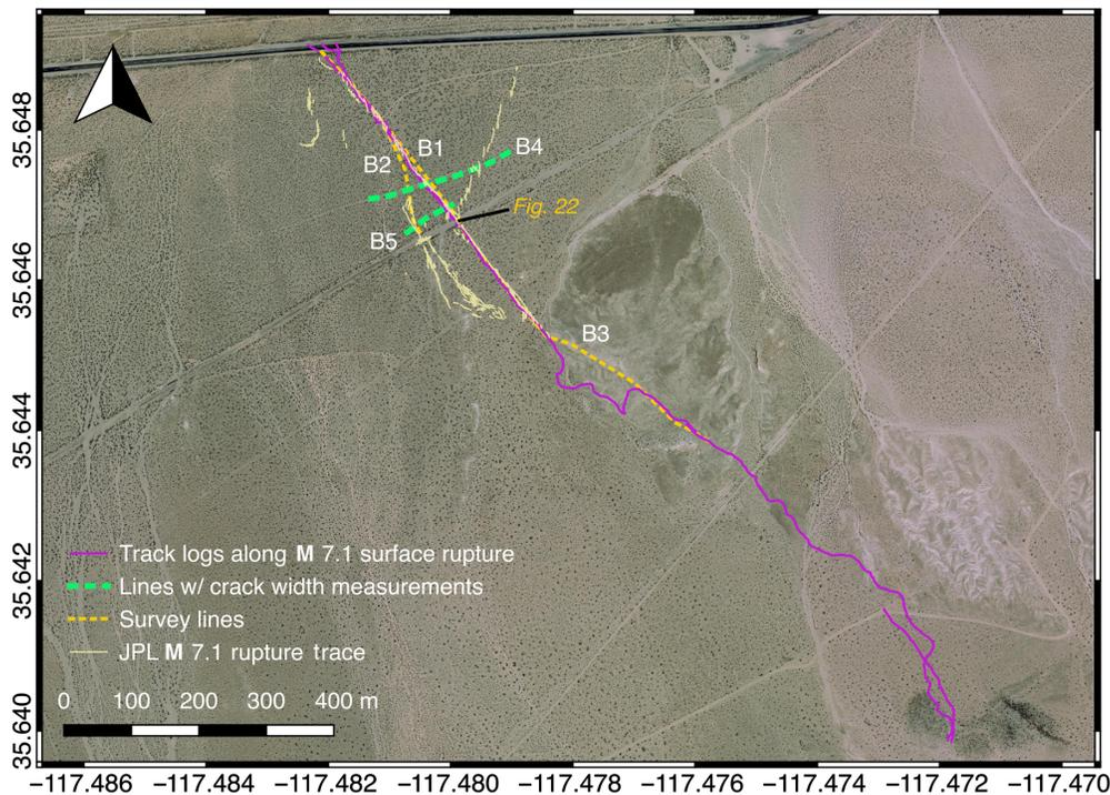
**Figure 4.** Map showing locations of measured ground cracks at location where **M 7.1** fault rupture crosses highway 178 (Stewart *et al.* 2019). The color version of this figure is available only in the electronic edition.
