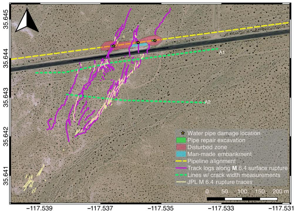
**Figure 3.** Map showing locations of measured ground cracks at location where **M 6.4** fault rupture crosses highway 178 (Stewart *et al.* 2019). The color version of this figure is available only in the electronic edition.
