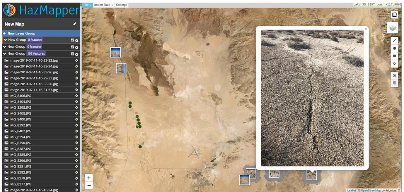
into a collection titled “M 6.4 Fault Rupture—UAV Survey.” Data products available for each processing batch from this mission include (1) a DSM in .tif format, (2) an orthomosaic in .tif format, (3) a point cloud in .las format, and (4) a folder for each point cloud created using the Potree converter in DesignSafe. Figure 9 shows a point cloud for the M 6.4 surface rupture at a location where the road is being repaired.
