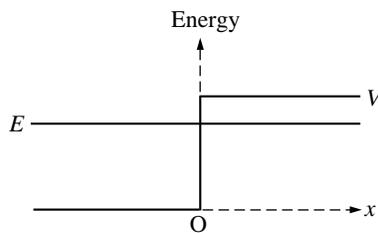
31. An electron with energy  $E$  and momentum  $k\hbar$  is incident from the left on a potential step of height  $V > E$  at  $x = 0$ . For  $x > 0$ , the space part of the electron's wave function has the form
