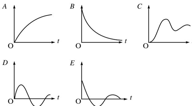
8. Which graph represents the potential drop across the resistor as a function of time in an inductance-resistance circuit?
