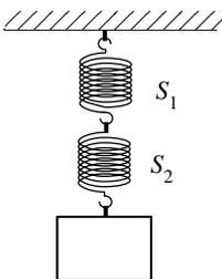
2. Two springs,  $S_1$  and  $S_2$ , have negligible masses and the spring constant of  $S_1$  is  $1/3$  that of  $S_2$ . When a block is hung from the springs as shown above and the springs come to equilibrium again, the ratio of the work done in stretching  $S_1$  to the work done in stretching  $S_2$  is
