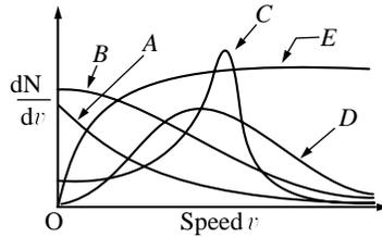
22. Which of the curves in the graph above best represents the distribution of speeds of the molecules in an ideal gas at thermal equilibrium?
