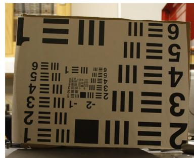
Fig. 4. An image of the test chart, taken at  $f/8.0$ . The data plotted in Fig. 5 is taken by sampling a horizontally oriented row of pixels across vertically oriented targets within this image.
